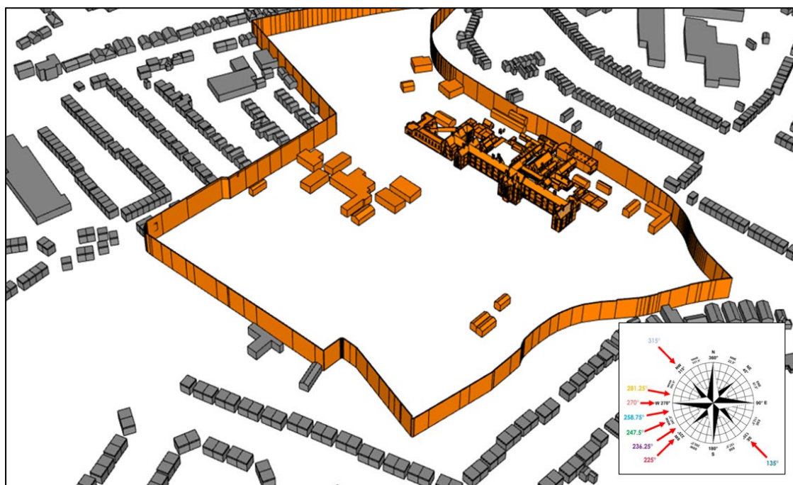
Figure 16.15: 3D model for the CFD wind analysis (Baseline existing environment).
