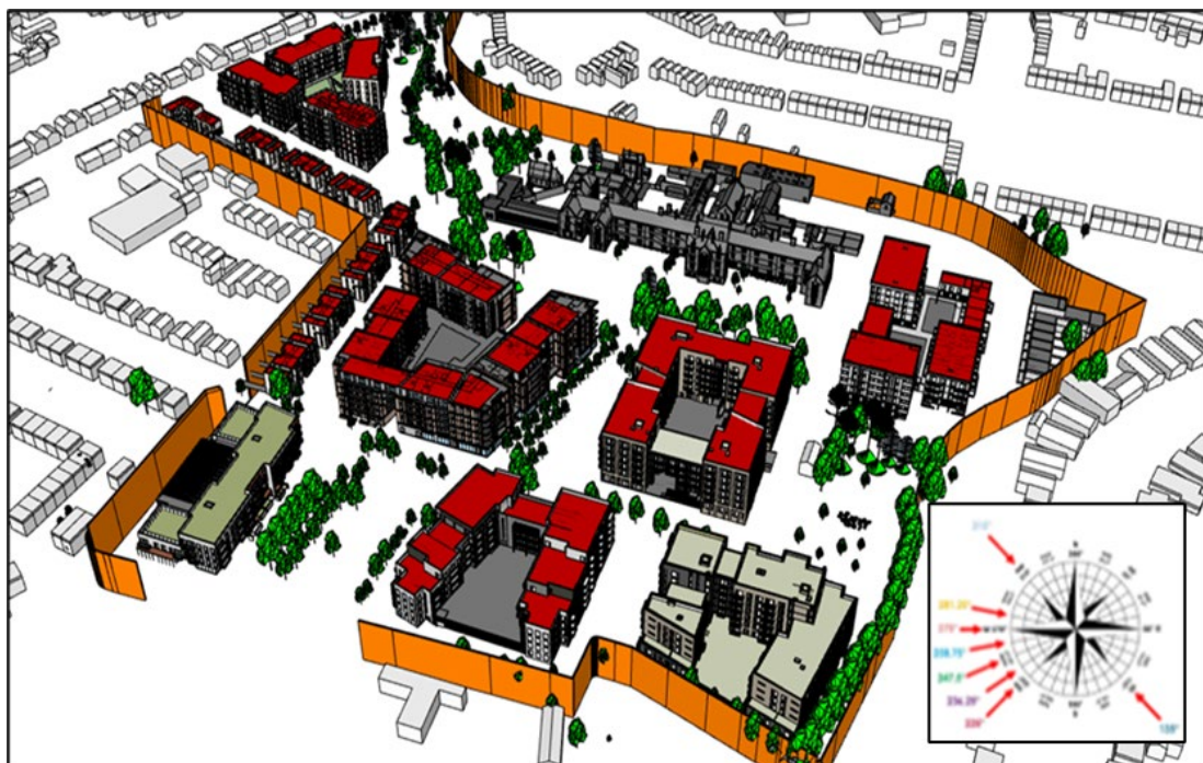
Figure 16.35: 3D model for the CFD wind analysis (proposed development within the existing environment and proposed landscaping included).
