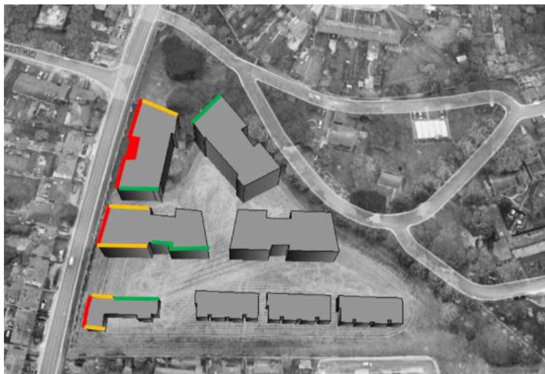
Figure 12.13: Designation of Predicted Noise Levels for Each Façade.
