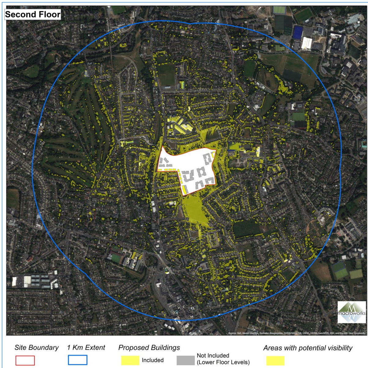
Figure 13.11: Zone of Theoretical Visibility (ZTV) map based on Digital Surface Model (DSM) data generated for the lowest 2 storey elements.
