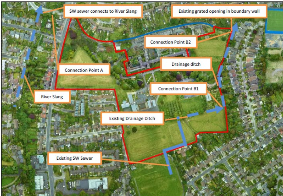
Figure 10.2: Aerial view of the site with water drainage indicated (Source: BMCE, 2022).
